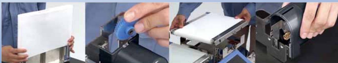
Replacing a belt
